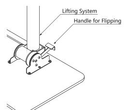
Insert the base to lifting system, fasten it with the nut by hand, and three screws by hex key.
